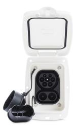
The Combined Charging System (CCS) is a standard for charging electric vehicles. It can use Combo 1 or Combo 2 connectors. These two connectors are extensions of the IEC 62196 Type 1 and Type 2 connectors, with two additional direct current (DC) contacts to allow high-power DC fast charging.
