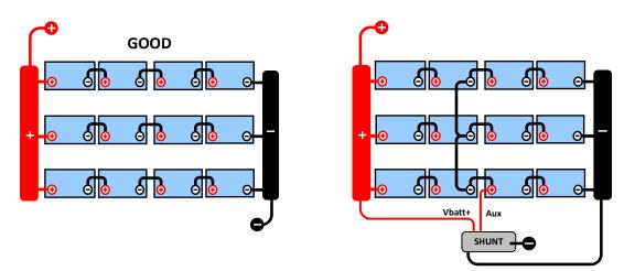
In an unmonitored battery bank the midpoints should not be interconnected, one bad battery bank can go unnoticed and could damage all other batteries.
