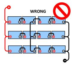
Due to the voltage drop over the positive and the negative cables the midpoint voltage are not identical.
