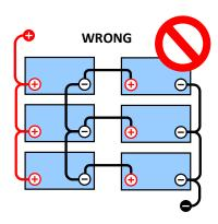
Due to the voltage drop over the positive and the negative cables the midpoint voltage are not identical.
